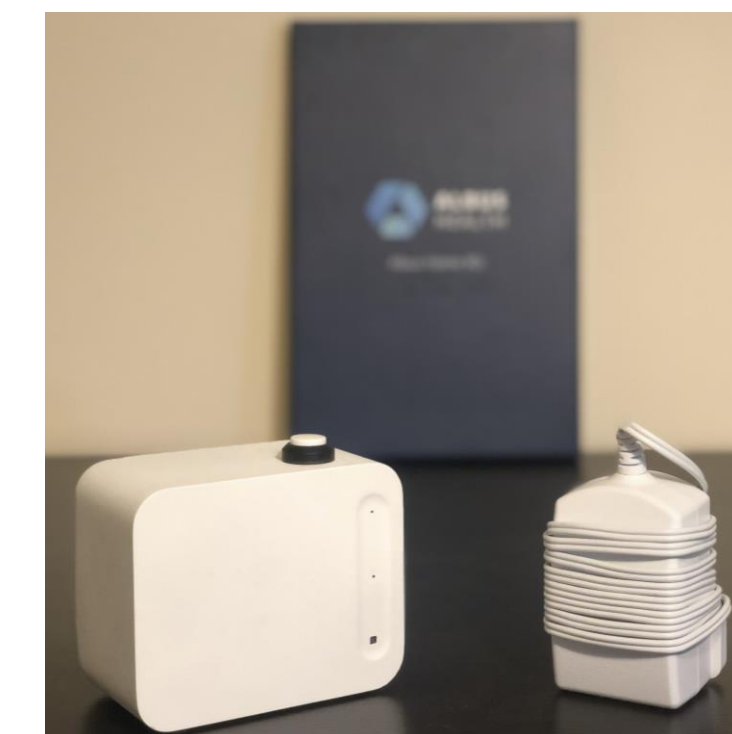
Figure 4: The plug-and-play Albus Home RD wirelessly captures automated RR, cough and air-quality metrics.
