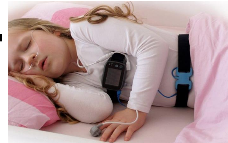
Figure 2: The current gold-standard, wearable PSG (SOMNOtouch™ RESPIRATORY, Somnomedics).
